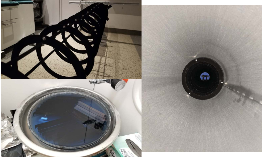
Figure 4.7: Images of the copper oxide procedure and final parts. Upper left shows the final assembly of the baffles structure. The right image shows this assembly being slid into the solenoid tube. The lower left shows the struts of the baffle structure mid-oxidation - the light colored ones were just added to the solution and hadn't yet formed an oxide layer.
