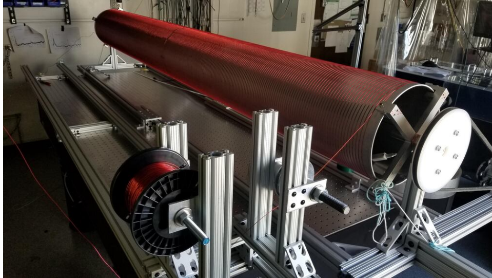
Figure 4.5: The 'rotisserie' that was built to wind the solenoid on a 10ft aluminum tube. The tube was mounted on each end to bearings, and the right side was attached to a drive belt and a car window motor. The UHV kapton wire was mounted to a track that could slide along as the coil was wound. Imaged here was our test winding before winding the real-deal solenoid, so we didn't need to maintain UHV cleanliness.
