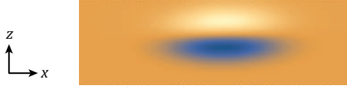
Figure 5.4: Thermally Dephased Signal. Numerical integration of the signal over the thermal velocity distribution and beam profile shows a reduction in contrast due to the thermal motion of the atoms.
