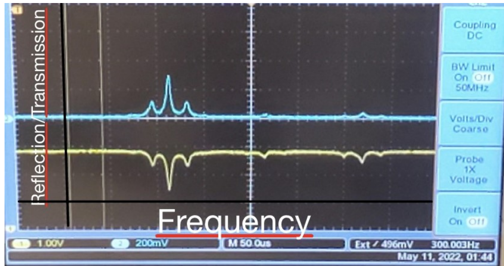
Figure 4.4: Carrier and Sidebands: The effect of frequency modulating the laser with and RF signal. The blue signal is the transmission through the cavity, and the yellow signal is the reflection.
